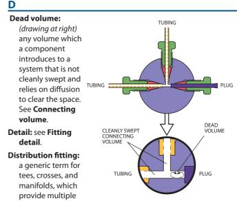
access points to "distribute" a gas or liquid through a system. *CAUTION!* Using a distribution fitting in reverse to coalesce multiple streams may create dead volume. Special manifolds are available for this application.
