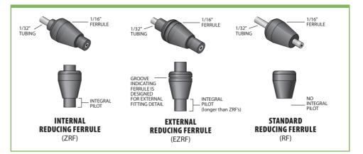
dead volume fitting. A single groove indicates that the ferrule is for use in an external detail.
