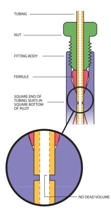
**Zero volume:** while often used interchangeably with zero dead volume, it ideally describes a fitting design in which there is no internal volume, such as a through-type union designed to butt-fit two pieces of tubing.
