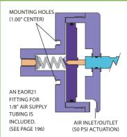
ULTRA-HIGH PRESSURE 40K ON/OFF AND PRIME/PURGE VALVES 40,000 psi valves .... p 65
