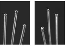
AVOID UNEVEN ENDS AND BURRS, DUE TO FILES (L) AND PLIER CUTS (R)
