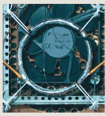
**RESISTIVELY-HEATED COLUMN** installed in traditional column oven
